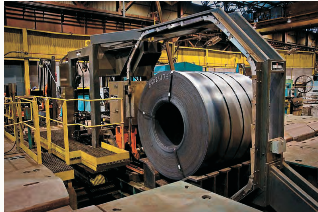
High speed dual head circumferential strapper for hot coils @ 800° F
