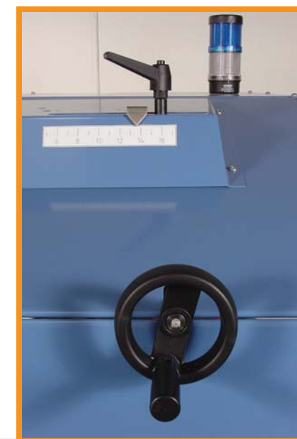
Single quick-release handle makes for quick backstop changes
