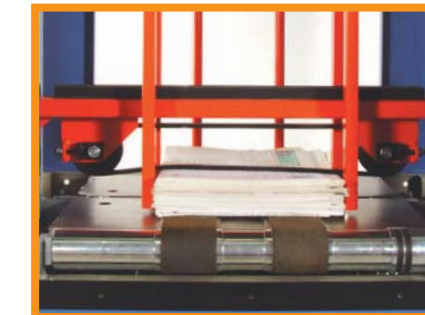
Bundle is tightly secured prior to strap placement making for a nice, presentable package to the carrier force
