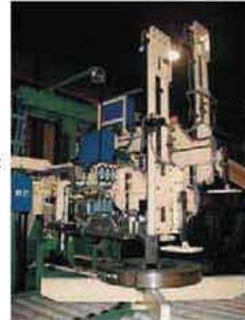
Lift and turn tables eliminate damaged coil edges
