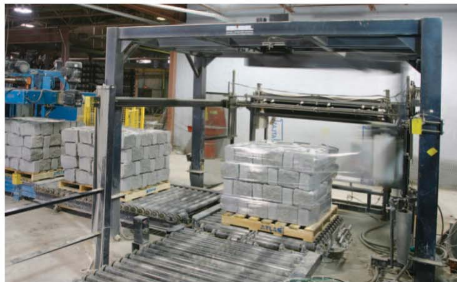
Samuel SRA 650 Rotary Arm Stretch Wrapper with top sheet dispenser.
