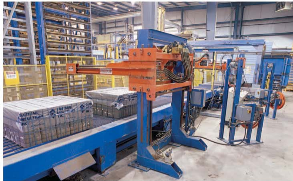
Horizontal and Vertical Strappers with M100 heads and automatic top sheet dispenser.
