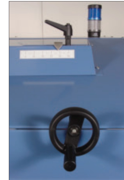
Single quick-release handle makes for quick backstop changes
